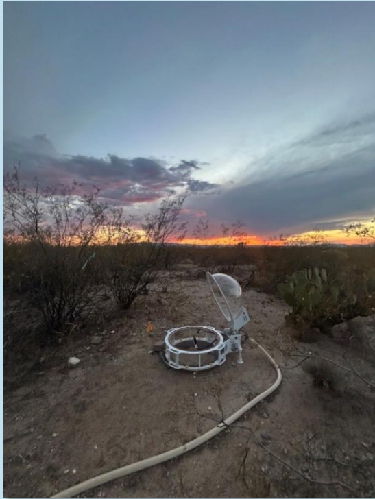
H_2 soil flux chamber (1 of 8) presently deployed near the NEON tower
